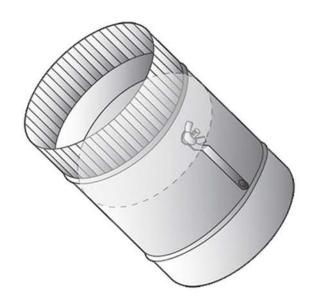
It is formed from rust-resistant, heavy gauge, galvanized steel and installs in seconds. The Rapit will penetrate and secure to round or rectangular damper blades and up to 24 gauge steel. It has fully retractable bearings of zinc alloy, threaded to accept a 5/16"-18 wingnut and a handle that indicates the damper position.
