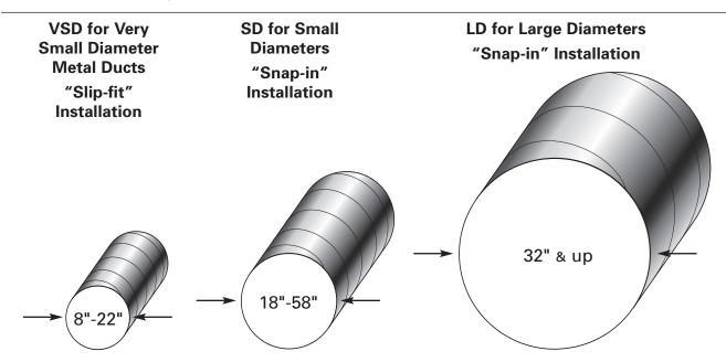
Minimum to maximum metal duct inside diameter ranges vary by insulation thickness. Please refer to the tables in AHS-361, AHS-362 and AHS-363 for specific applications for 1", 11/2" and 2" thick insulations, respectively.
