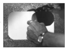
3. Insert door into opening at an angle and tighten knobs.
