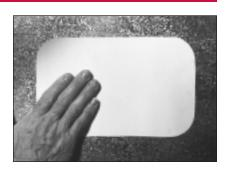
2. Opening can be cut with hand-held plasma cutter or by conventional methods.
