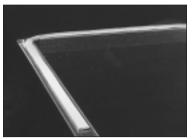
13. Systems '25' and '35' use 5/8" Ductmate 440 Gasket Tape. Start applying halfway between duct corners. Position in center of Ductmate angle as in photo.
