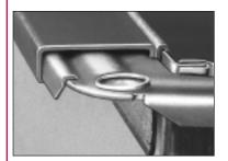
9. The duct must be seated all the way into the Ductmate angle in order to penetrate the integral mastic sealant and avoid leakage. The corner of the duct *MUST* protrude beyond the Ductmate corner piece.
